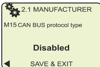
**M15:** With this parameter it's possible to activate the reading of some functioning data for motors VOLVO-IVECO-DEUTZ. It is also foreseen the reading of parameters which: motor revolutions (rpm), motor temperature, oil pressure and motor high temperature bulb. Information on CAN BUS line have the priority on the acquisition of the respective values by external sensors that are directly connected with IdroMOP.
